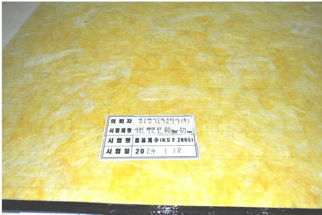
[PHOTO 1] Test specimen arranged in reverberation room
